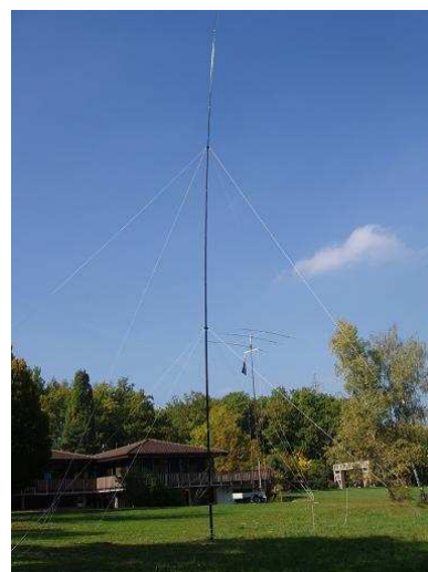
80m vertical and beam in the back
